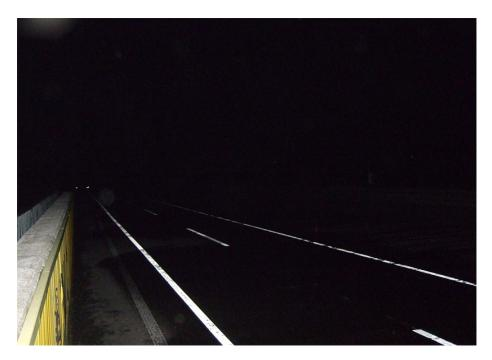
Figure 2. Marking material II, with additional wet reflectivity (picture shows wet track)
